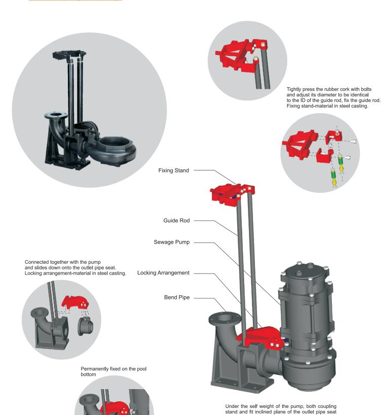
are tightly wedged and then closely fitted with the sealing surface of the seat to finish automatic coupling installation. The pump will automatically separate from the outlet pipe seat when lifted. Bend
